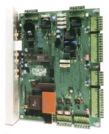
he ST5000 BASeStation is the latest Building Access Security series designed and manufactured by Sierra Technology. Based on the successful and popular ProxStation and Starprox series of single door access control systems, the new and exciting ST5000 BASeStation Series is incorporated onto a single integrated processor board with built-in power supply and control module, card read interface electronics as well as lock control and monitoring circuitry.
